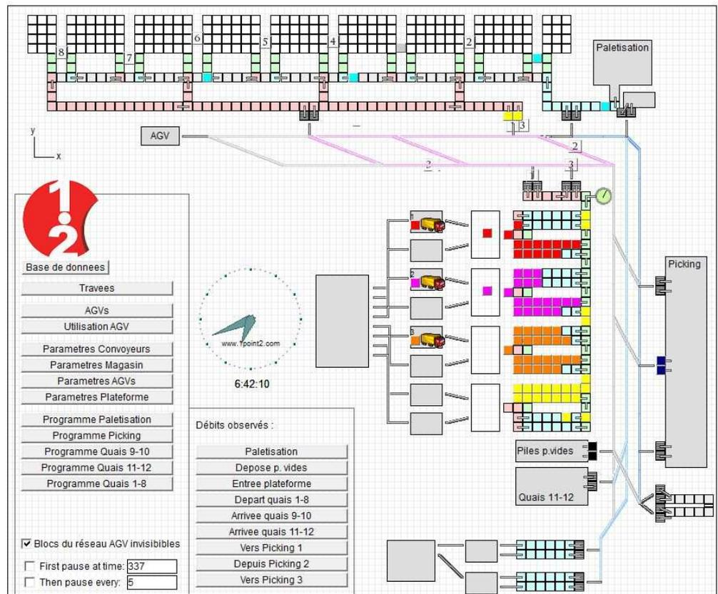
The dynamic study first focused on developing a warehouse model in order to find the optimal dimensioning for pallets transportation equipments:
